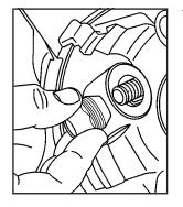
10. Put the wheel nuts back on with the rounded end of the nuts toward the wheel. Tighten each wheel nut by hand. Then use the wheel wrench to tighten the nuts until the wheel is held against the hub.
